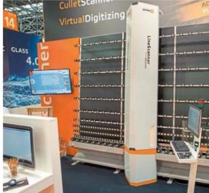
**Testing** the overall warpage of the glass is a further development of the LineScanner.
