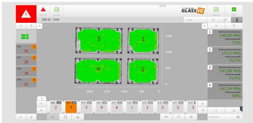
Figure 1: The thematically prestressed glass products are scanned and evaluated on the screen.
