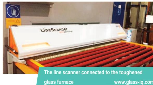
systems to be determined using the scanner. The Flintermann GmbH and Egger Glas GmbH companies also made an essential contribution to its realisation. The hardly surprising result: the characteristics of the anisotropies are to a large extent system-specific.
